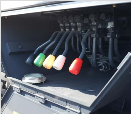
支腿伸缩软轴操纵 Soft shaft operation for outrigger telescoping
